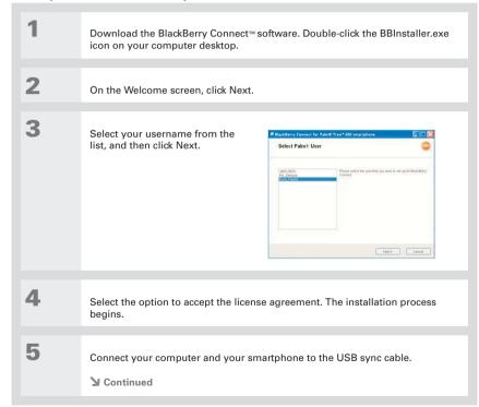
Leave your computer and your smartphone connected to the sync cable after synchronising in step 6, because you need to synchronise again later in the installation process.
